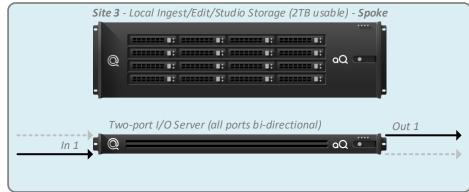
All ports are bi-directional SDI with embedded audio. This configuration provides a total of 8 ports at the Hub and 2 ports in each of the Spoke sites. Half are nominally configured as recorders and half as players, but any allocation can be switched on-the-fly. Alternatively, the number of I/O servers could be decreased or increased dependent upon the exact requirement.
